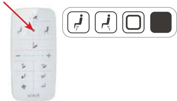
**Stand-by Mod:** Stand-by mode can be adjusted by pressing stop button on the left side of the WC (when facing the WC) for 3 seconds. All functions are disabled. Only water temperature controller unit is turned on to keep water temperature above 18°C. When the light on the left hand side of the WC is turned Off, the WC is in Standby-Mode.
